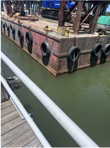
Figure 7. May 16, 2026 (F04, F14). Left: the crane barge's hull and tire fenders a few feet off the pier's outboard pile line and facing the piles, with a TADANO crane and generator aboard; hull marking ending 124 B. Right: two barges moored at the end of the pier with girder erection in progress behind them.
